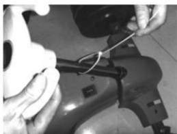
18. Bind the wires on the pole.
