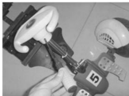
17. Pull out the orientation pole, assemble the steering wheel and adjust the height.
