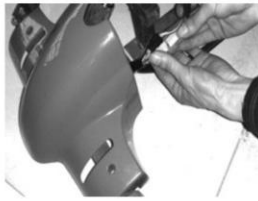
14. Connect the steering wheel connectors.
